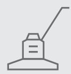
IN ORDER TO SMOOTH THE SURFACE, TROWEL WITH A MECHANICAL TROWEL (HELICOPTER) OR OTHER. **CURE FOR THREE DAYS AND CUT** WITHIN 48 HOURS.
