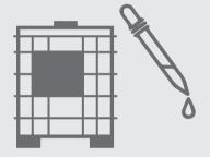
ADD TOPTEC® AT THE BATCHING PLANT WITH THE TEMPERING WATER TO THE **CONCRETE MIXTURE OR TO READY MIXED CONCRETE BATCH AT SITE.**
